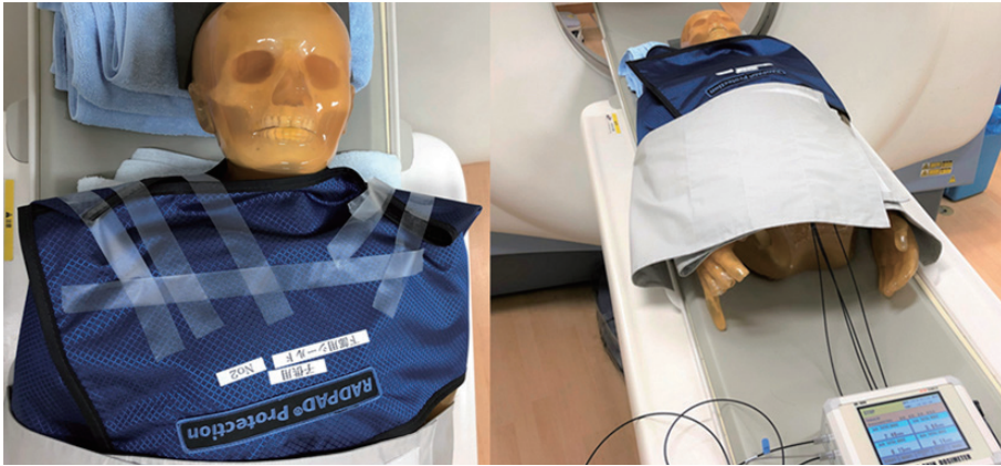
Fig. 2. Measurement setup with the RPS. Measurements were conducted with the RPS encircling the body from the neck to the chest.
