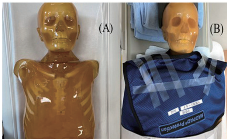
Fig. 1. Whole-body human-equivalent phantom (Whole Body Phantom PBU-10; Kyoto Kagaku, Kyoto, Japan) without (A) and with (B) the RPS.
